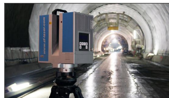
Figura 7. Laser scanner
